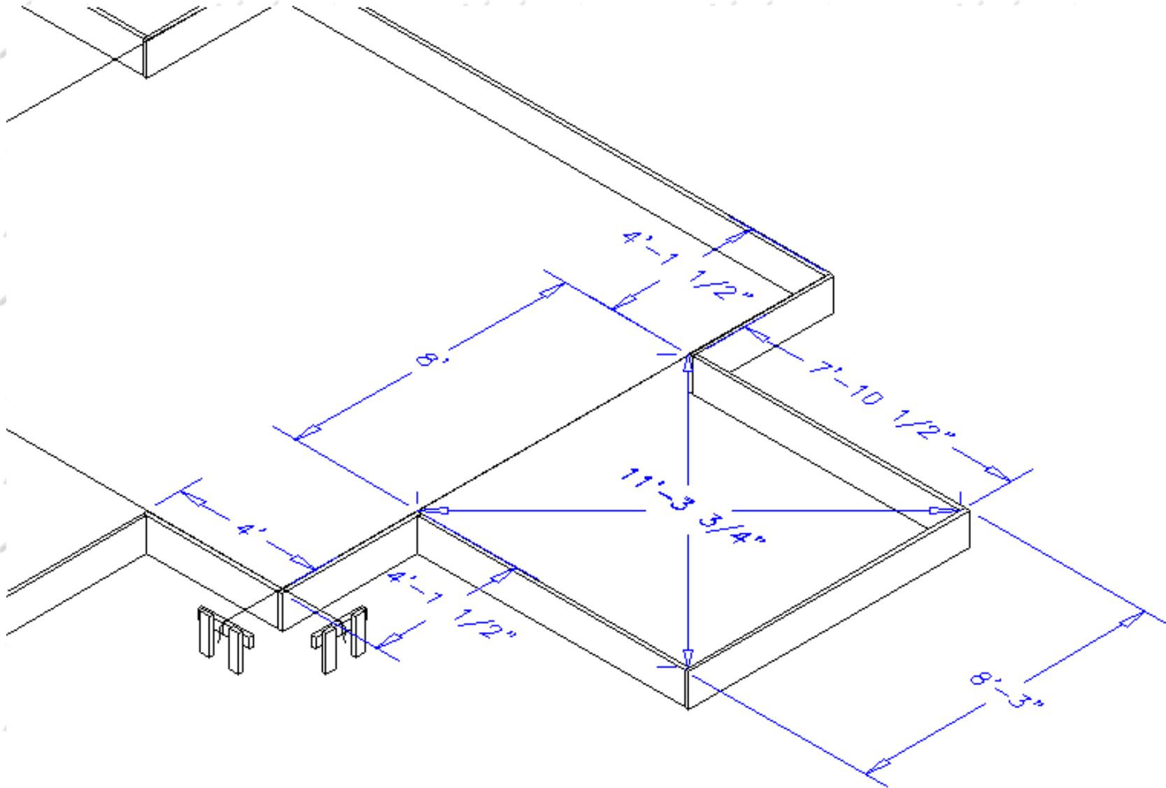
5. Place stakes with kick braces every 2' to 4'. Level forms starting in the back corner and working around the perimeter. Nail boards to stakes.
